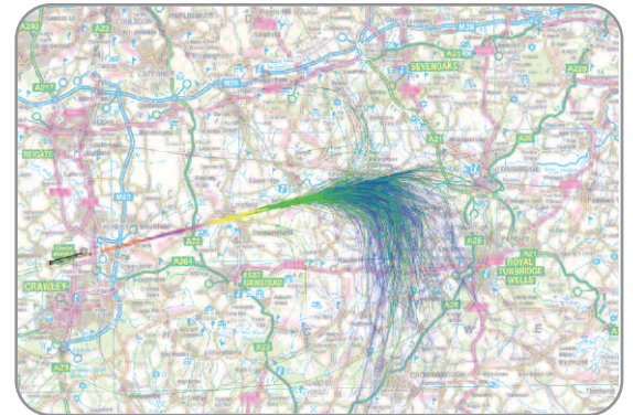
Figure C14 Colour by height plots of westerly (23:30-06:00) arriving aircraft to 4,000ft for July 2008
