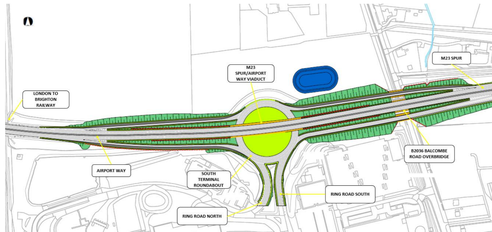
Figure 5: M23 Spur/Airport Way Flyover (50mph) Option 1b Concept Layout
