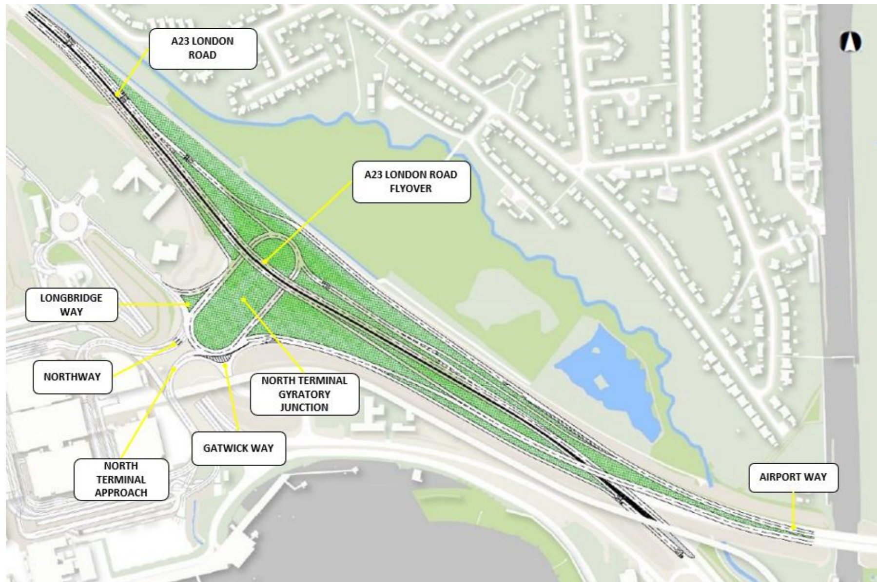
Figure 13: Option 1a North Terminal Grade Separated Junction Concept Layout.
