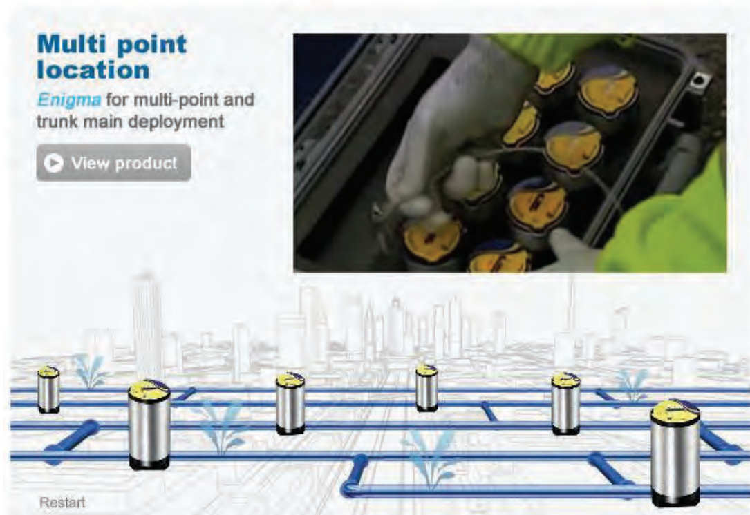
Figure 8-7 : Acoustic noise loggers/correlators (Source: Primayer)
