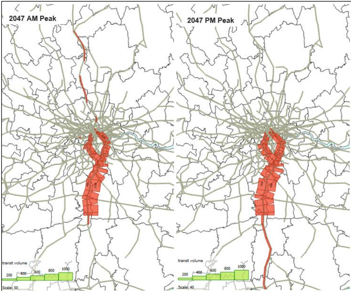
Diagram 12.4.4: 2047 flow change between future baseline and With Project - AM and PM peak periods (0700-0900 and 1600-1800)
