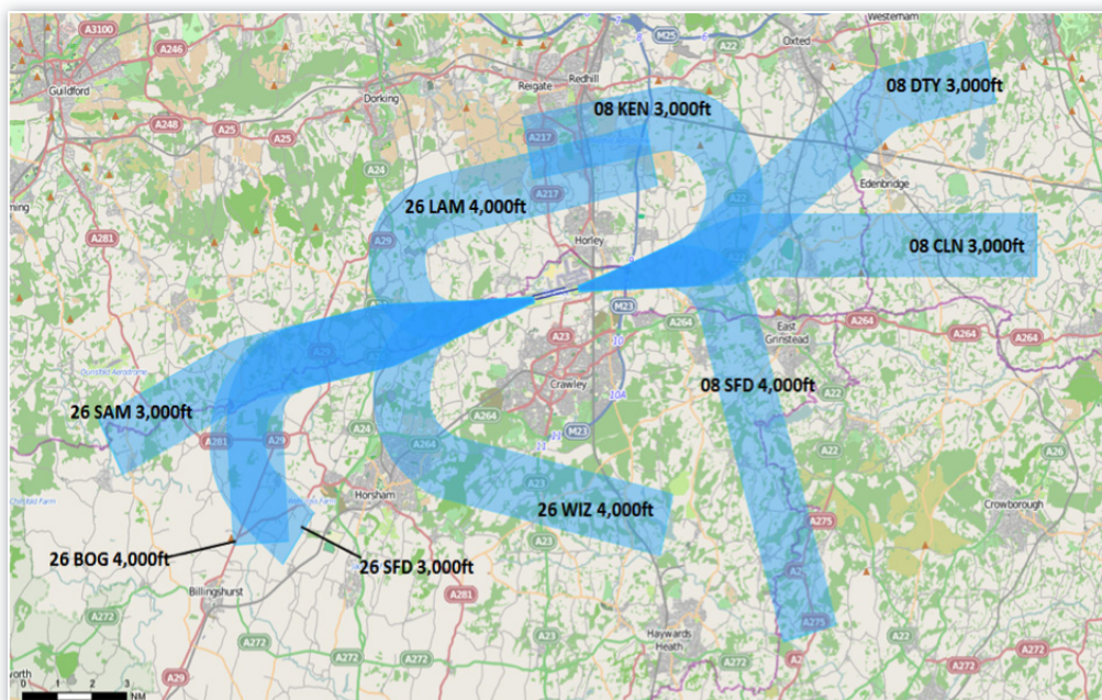
FIGURE 10 – MAP OF THE NOISE PREFERENTIAL ROUTES AT GATWICK AIRPORT USED BY DEPARTING AIRCRAFT WITH MINIMUM ALTITUDE FIGURES
